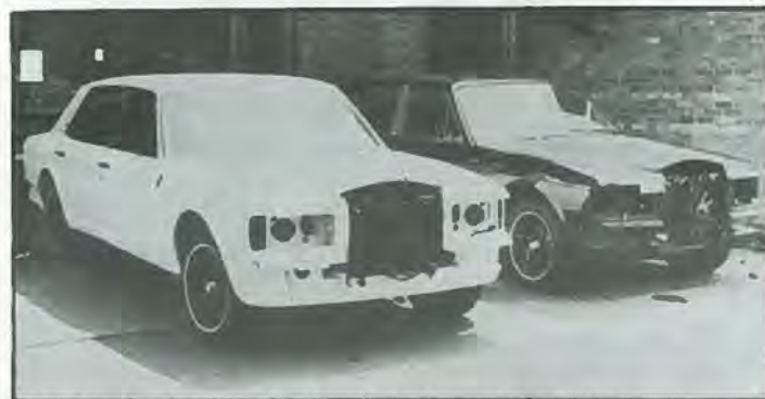
This is how the cars go out on road test. Only when any faults which come to light during the test have been rectified, and the car given a final coat of paint, will it be allowed to gain the famous radiator grille.
